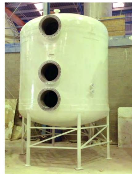
Filters tank Vertical sand
