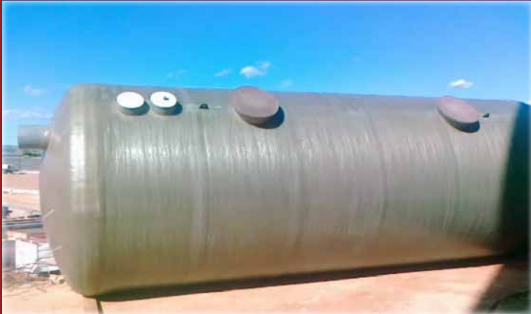
Hydrocarbon separation plant
